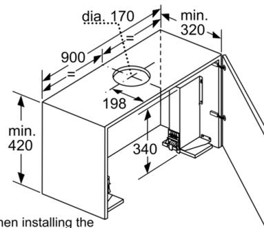
When installing the 90 cm telescopic hood in a 90 cm wide wall-hanging cupboard, the mounting kit is required. The two mounting brackets are screwed onto the right and left of the kitchen unit. Installation in accordance with template.
