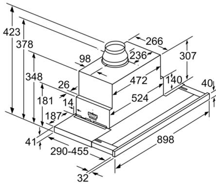
Depth of the filter drawer can be adjusted
