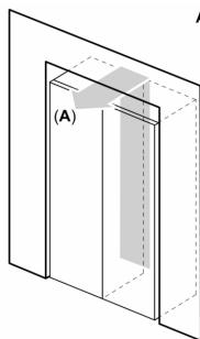
A: Odvod vazduha  $\geq 200 \text{ cm}^2$
