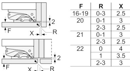
The gap dimensions recommended in the table must be adhered to in order to ensure that appliance doors do not collide with anything when they are opened, and to avoid causing damage to kitchen units.
