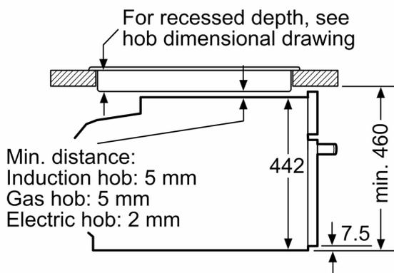
If the compact appliance will be installed underneath a hob, the following worktop thicknesses (including substructure if necessary) must be taken into account.
