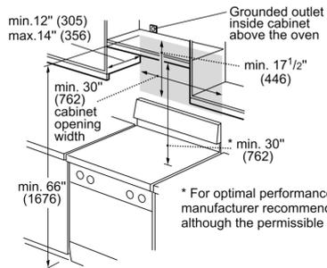
\* For optimal performance and reliability, the manufacturer recommends a clearance of 33"-36", although the permissible clearance must be at least 30".
