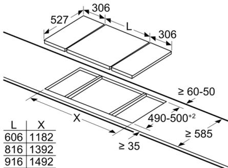
When installing two Domino units right next to a hob, two assembly kits (HEZ394301) are required.
