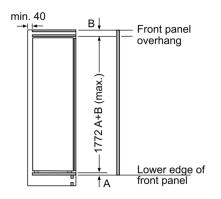
measurements in mm
