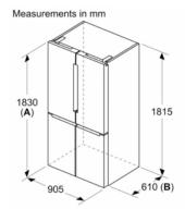
A: Front is adjustable 1830–1847 mm, with front levelling feet fully extended
