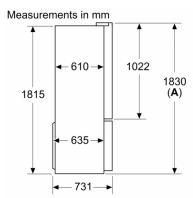
**A:** Front is adjustable 1830–1847 mm, with front levelling feet fully extended
