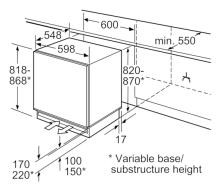
Space for electrical connection next to the appliance on the left or right-hand side. Ventilation space in the base. measurements in mm
