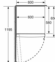
measurements in mm
