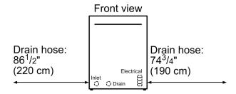
The electrical junction box and water inlet are at the front of the appliance, the drain at the rear.
