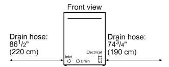
The electrical junction box and water inlet are at the front of the appliance, the drain at the rear.
