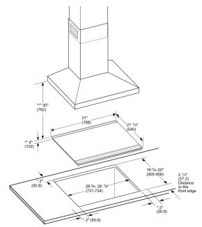
mum distance between the cooktop surface and er edge of the exhaust hood. Dimensions in inches (mm)
