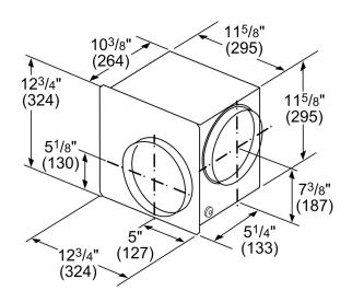
measurements in inches and (mm)
