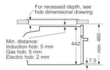
measurements in mm
