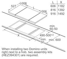
Measurements in mm
