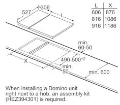
Measurements in mm
