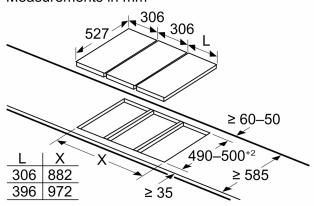
If two or more elements are installed right next to one another, one or several installation kits are required (2 elements 1 installation kit, 3 elements 2 installation kits, etc.)
