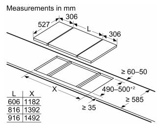
When installing two Domino units right next to a hob, two assembly kits (HEZ394301) are required
