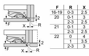
The gap dimensions recommended in the table must be adhered to in order to ensure that appliance doors do not collide with anything when they are opened, and to avoid causing damage to kitchen units.
