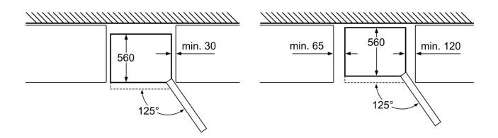
Measurements in mm
