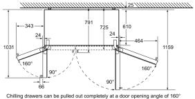
illing drawers can be pulled out completely at a door opening angle of 160° measurements in mm
