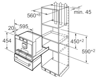
The fully automatic espresso machine can be fitted above a warming drawer. An intermediate floor is not required.
