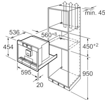
An installation height >950 mm makes it difficult to fill the containers for beans and water which are fitted on the top.
