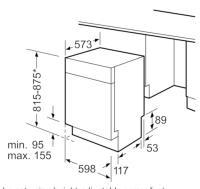
\* Can be set using height-adjustable screw feet Base height (when appliance height is 815) - 95 mm Base height (when appliance height is 875) - 155 mm
