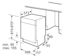
\* Can be set using height-adjustable screw feet Base height (when appliance height is 815) - 95 mm Base height (when appliance height is 875) - 155 mm measurements in mm
