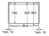
\* If the appliance is placed next to a cooker, the side distance must be 10 mm minimum.
