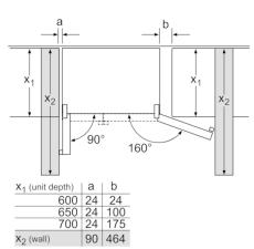
measurements in mm
