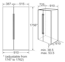
measurements in mm
