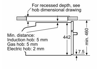
measurements in mm
