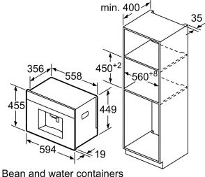
are removed from the front. Recommended installation height 95-145 cm.
