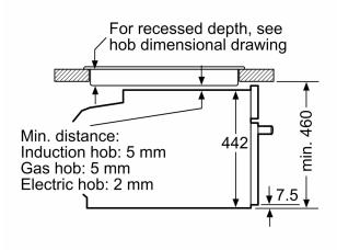
measurements in mm
