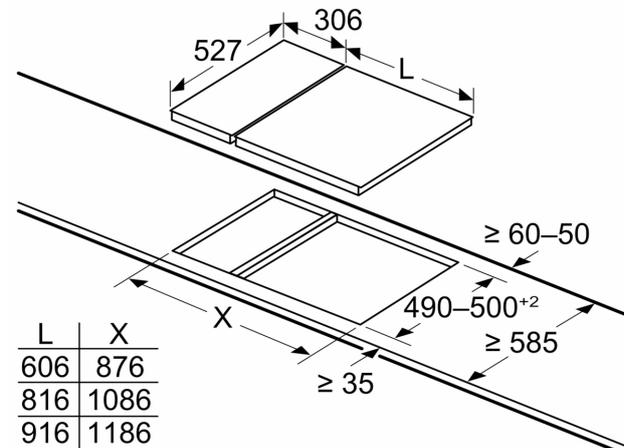
When installing two Domino units right next to a hob, two assembly kits (HEZ394301) are required
