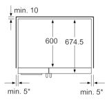
\* If the appliance is placed next to a cooker, the side clearance must be 30 mm minimum.
