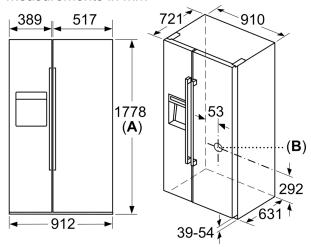
**A**: Front is adjustable from 1769 to 1784 **B**: Water connection to the appliance
