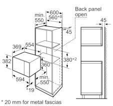
measurements in mm
