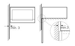
Measurements in mm
