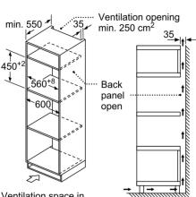
Ventilation space in the base min.  $50 \text{ cm}^2$
