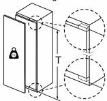
Fitted kitchen unit doors that exceed the permissible weight may cause damage and result in functional impairment of the hinges.
