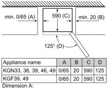
In models with vertical integrated handles, in order to open easily, a minimum distance of 65 mm is needed.
