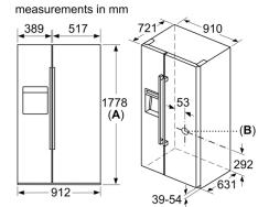
A: Front is adjustable from 1769 to 1784 B: Water connection to the appliance
