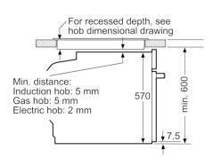
measurements in mm
