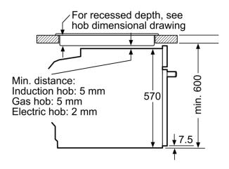
measurements in mm
