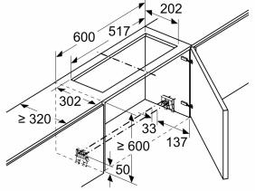
Not possible to use a circulated air kit for cupboards with transverse cross-members (lifting doors)
