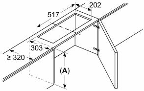
Not possible to use a circulated air kit for cupboards with transverse cross-members (lifting doors)
