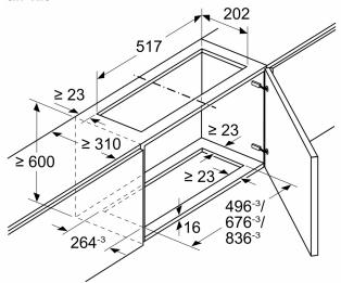
Measurements in mm Installation of telescopic hood with circulated air kit and lowering frame
