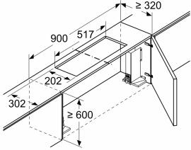
Not possible to use a circulated air kit for cupboards with transverse cross-members (lifting doors)
