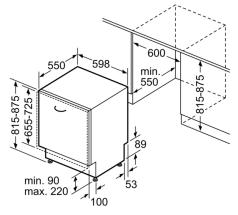
measurements in mm
