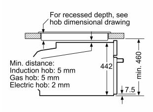
measurements in mm
