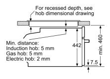
measurements in mm
