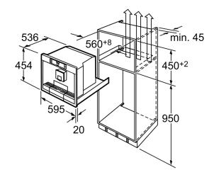
An installation height >950 mm makes it difficult to fill the containers for beans and water which are fitted on the top.
