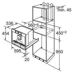
An installation height >950 mm makes it difficult to fill the containers for beans and water which are fitted on the top.
