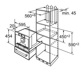
The fully automatic espresso machine can be fitted above a warming drawer. An intermediate floor is not required.
