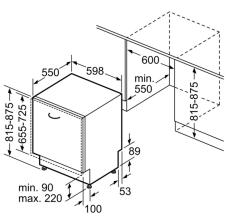
measurements in mm
