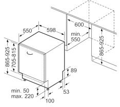
measurements in mm
