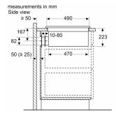
When installing directly against outer walls that are not insulated ( $\mu \ge 0.5 \ W/m^2$ °C), we recommend using partially or fully ducted recirculation configurations.
