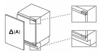
Fitted unit fronts that exceed the permissible weight may cause damage and result in functional impairment of the hinges
