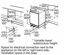
Measurements in mm
