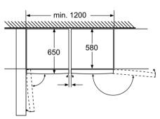
Drawers can be pulled out completely if the appliance is placed directly on a wall. measurements in mm
