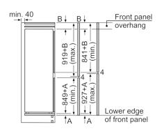
The specified unit door dimensions are valid for a door gap of 4 mm. measurements in mm
